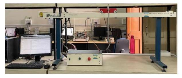
The Inverted Pendulum system setup provides a platform to test the developed control laws in realtime. The cart is equipped with a rotary metal shaft to which a free-turning pendulum can be attached. The Linear Servo Base Unit system has two encoders: one used to measure the cart's position and the other used to sense the position of the pendulum shaft.
