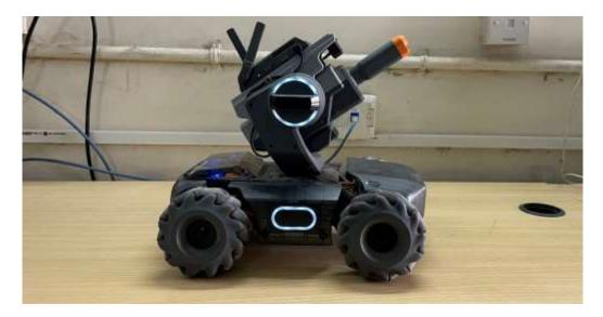
The Rob master set up with four Mecanum wheels allows the robot to move in all directions. Connected motors provide wheel motions as well as free sliding motion by 12 rollers on the wheel. This model is used as a testbench to apply different developed control strategies. Experimental applications are vision-based control, path tracking, obstacle avoidance, picking and placing objects with colour detection.
