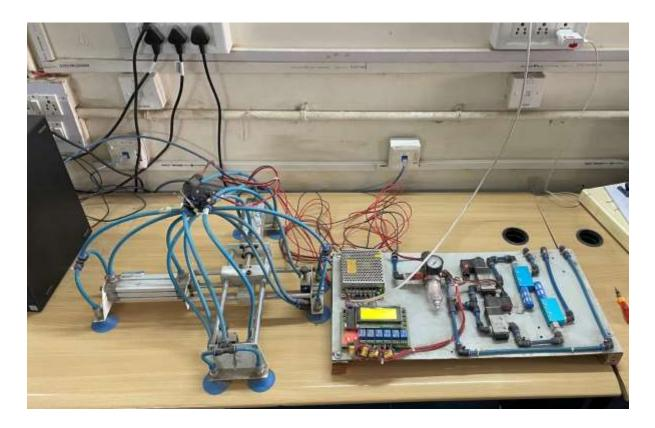
In this project, a prototype of a wall-climbing robot is developed. The user has to enter the dimension in terms of the X-axis and Y-axis. They are considering the fence as a two-dimensional Cartesian coordinate system (shown on 20\*4 LCD). After entering the dimension, once the user presses the start button robot will begin its journey towards the destination. The robot will first climb in the
