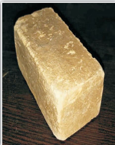
The brick made out of jarosite waste
