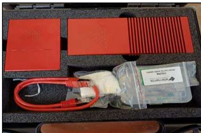
e-NPR 10MHz: Nanopore reader for detection of single-molecules with time resolution of 100 ns
