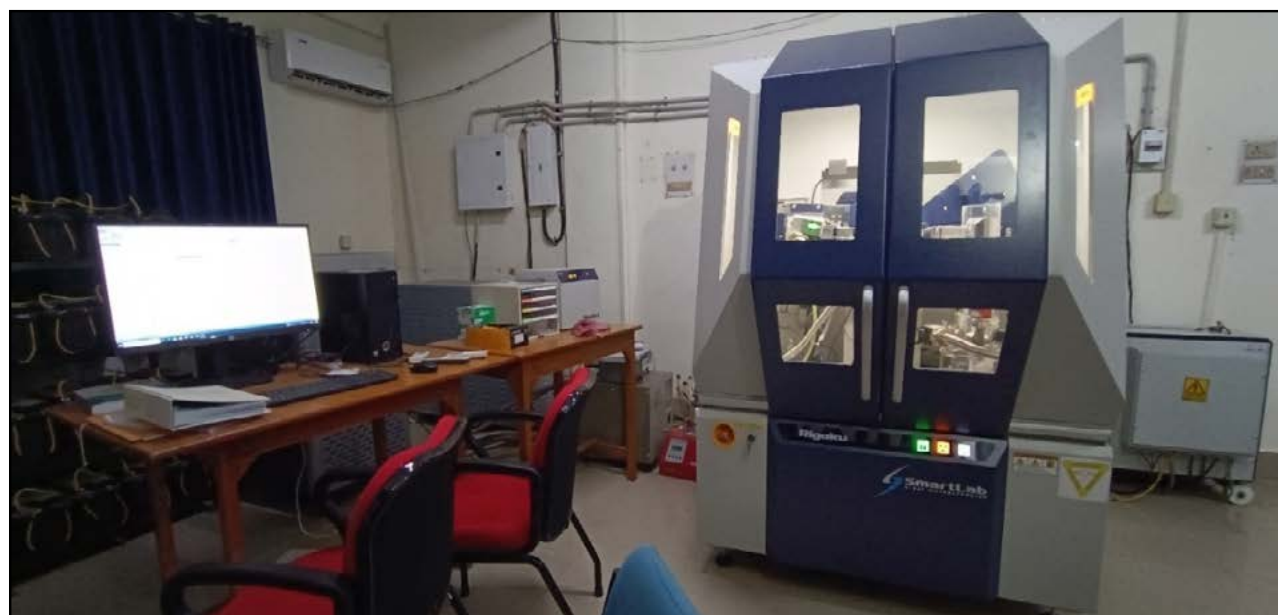
SmartLab 9kW X-ray Diffractometer (XRD) with Thin Film, Ultralow temperature (4K) and High Temperature (1500 OC)
