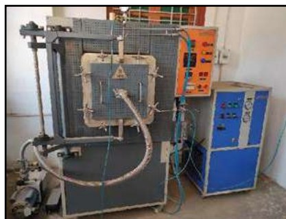
Machine: High Capacity Muffle Furnace Model: 1800 Deg. Celsius Make: AntsProslys
