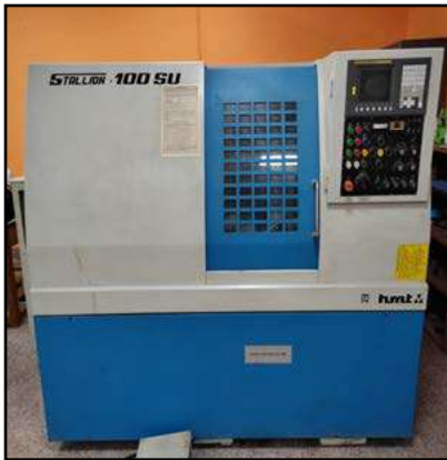
Machine: C.N.C. Lathe Machine, Model: Stallion -100 SU, Make: H.M.T.
