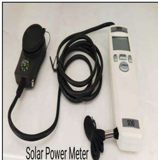
Solar Power Meter
