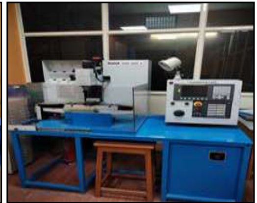
Machine: C.N.C. Milling Train Master, Model: VMC 200 T, Make: H.M.T.
