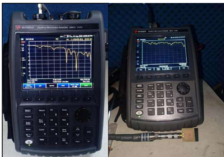
Handheld Vector Network Analyzer with measurement facility up to 44 GHz. The microwave characterization of the device under test can be performed at any location as the instrument is portable in nature.
