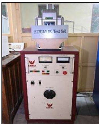
DC Dielectric Test set: 200 kV, 10mA, Phenix Technologies, USA
