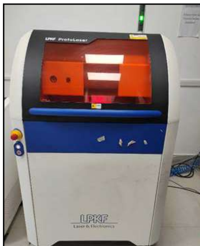
Machine: Multi Layered PCB Prototyping Model: PhotoLaser S4 Make: LPKF
