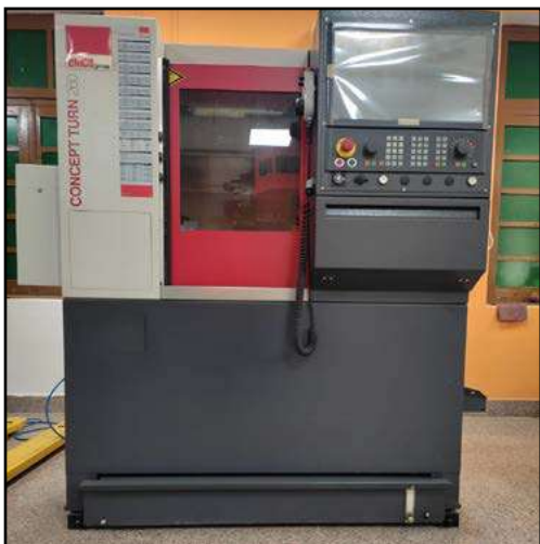
Machine: C.N.C. Lathe Model: Concept Turn 260 Make: EMCO Group
