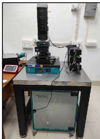
Machine: Raman Microscope / Spectrometry Model: Alpha300RA Make: WITec, Germany
