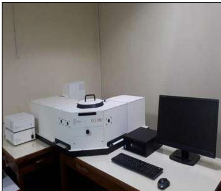
Photoluminescence (PL) measurement setup (F980) from Edinburgh Photonics, UK. This setup can provide PL from 200-800 nm
