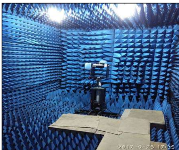
An “ anechoic chamber ” (“an-echoic” meaning non-reflective, non-echoing or echo-free) is a room designed to completely absorb reflections of either sound or electromagnetic waves. They are also often isolated from waves entering from their surroundings. ( Anechoic Chamber with 6 axis position for RF Characterization (up to 60 GHz) )
