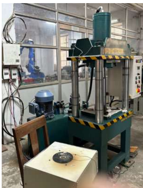
Cold/Hot Extrusion Machine Setup – 100 ton, Cost - 13.5 Lacs (for UG/PG Lab)
