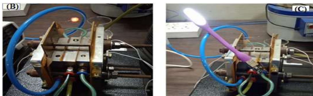
Fig. 2. Photographic view of (B) URPEMFC stack for hydrogen production in electrolysis mode and simultaneous power generation in Fuel cell mode showing LED light and (C) URPEMFC stack for hydrogen production in electrolysis mode and simultaneous power generation in Fuel cell mode showing array of LED light glowing with high intensity.
