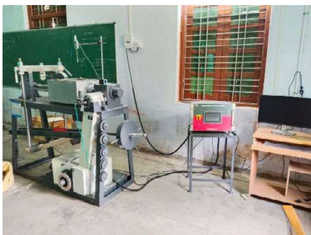
Large size direct shear automatic testing system for dump material
