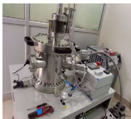
Figure 2. DC-magnetron sputtering units with four different targets and one magnetron source.
