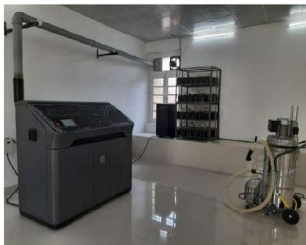
High Strength Colour Polymer 3D Printer Model HP-MJF-580
