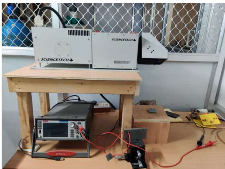
Solar Simulator (make: Science Tech) with Keithley source-meter
