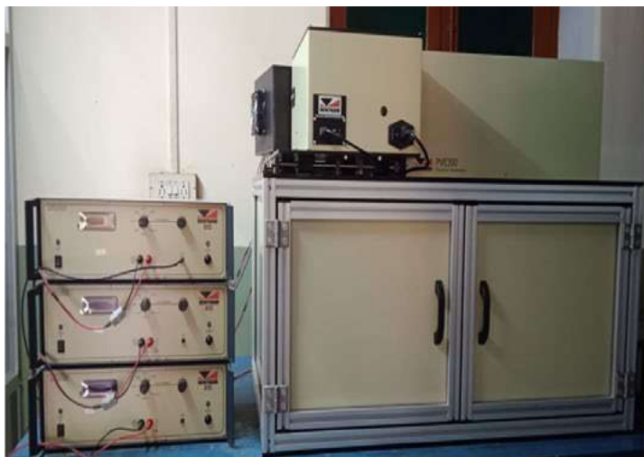
(A) Quantum Efficiency (QE) Set-up (make: Bentham) (B) Interior view of the QE
