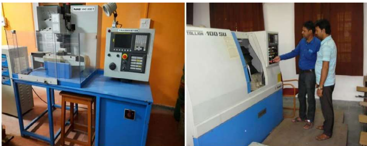
CNC Vertical Machining Centre - 3 Axis ( Train Master) and CNC Turning (Production Type)
