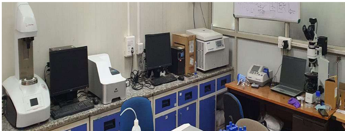
Fig.: Rheometer, Dynamic Light Scattering, ultracentrifuge, UV-Vis, Optical microscope (Biophysics and Nanotechnology Laboratory)
