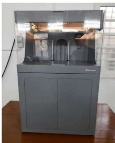
Markforged Model X-7 Fiber Composite 3D Printer
