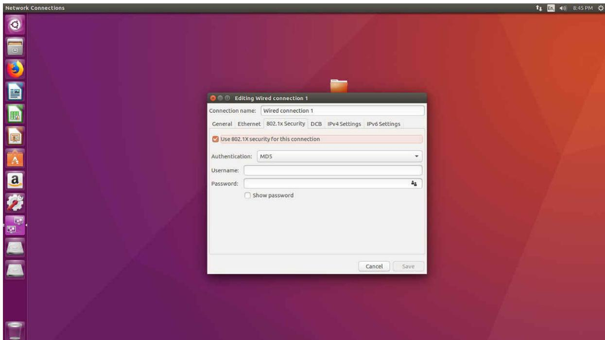
**Step 6.** Provide **PEAP** in Authentication and select **None** in C.A certificate.
